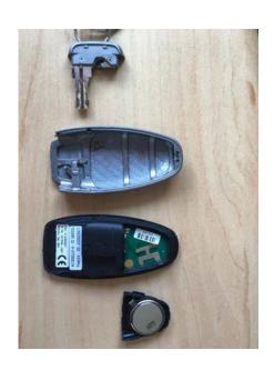
Step 3: Flick out the battery carefully ensuring the small silver clip which acts as a battery contact, remaining in place.
