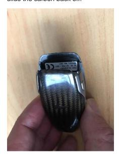
Step 2: Pry open the battery cover like above with a small bladed screwdriver or similar
