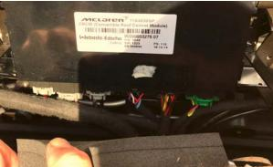
Pressing in the tabs on the retaining clips, ease out the connectors that need to connect to the roof module. (Refer to the manufacturer's instructions). Insert the car's connectors into the module wiring loom and vice versa.
