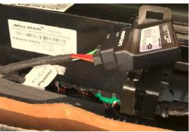
The additional cabling should be able to tuck in neatly within the space underneath the existing roof module.
