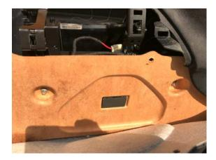
Loosen and remove the small bolts that retain the moulded panel to the framework. This will give you better access to the connectors at the bottom of the existing roof module.
